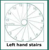
To allow for ease of installation and comfort in use, the opening in the floor should be finished no less than 50mm greater than the diameter to the stair; thus:
